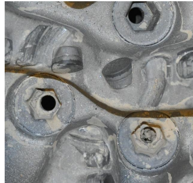
Bit 2: Post Drill after 566 ft.
