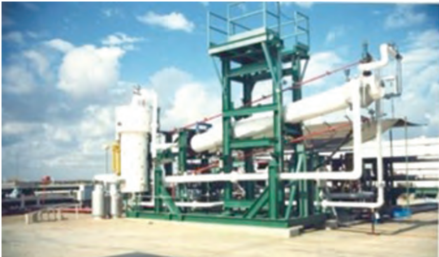
Figure 26. Heat Cycle Research Facility with the condenser at a 10-degree orientation
