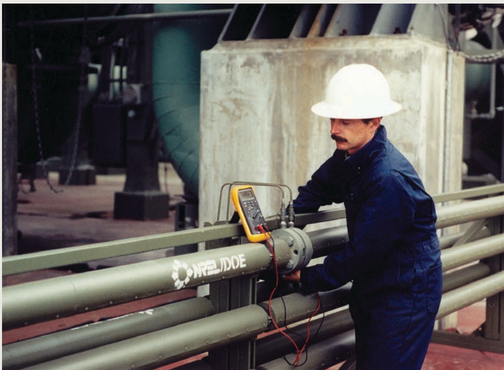
Keith Gawlick, of the National Renewable Energy Laboratory, field testing coatings at the Mammoth Pacific Geothermal Power Plant in the Sierra Nevada Mountains.
