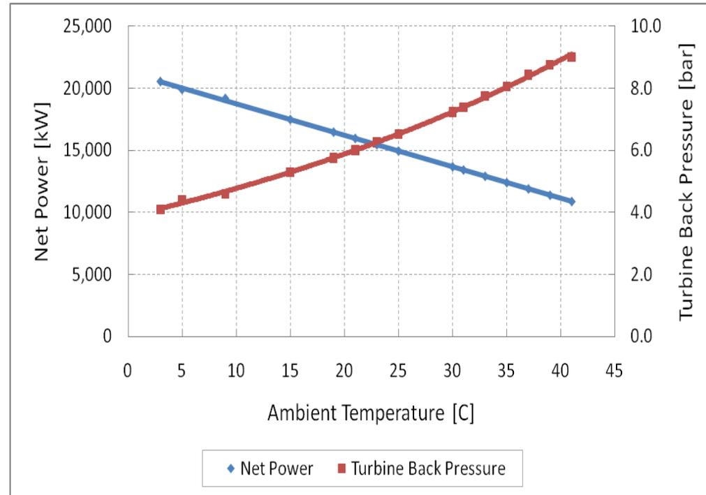
Study results for a 20-MW air cooled power plant simulation.
