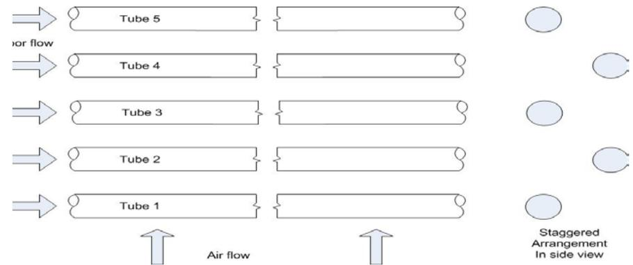
Geometry of heat exchanger
