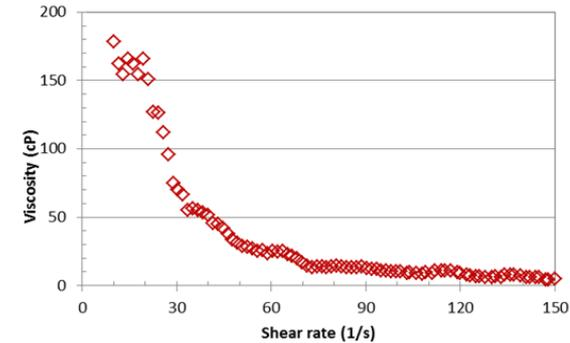
Shear thinning behavior at higher shear rates (190°C, 130 bar.)
