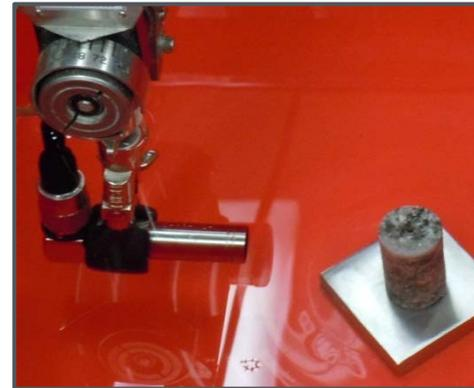
Missing section in rock sample shows up clearly as a (blue) low-amplitude return signal (red = highest amplitude)
