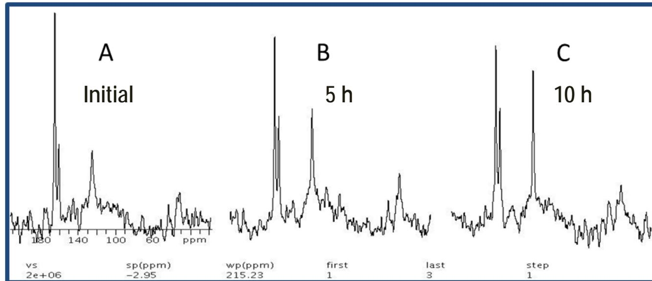
*In situ* time-resolved  $^{13}\text{C}$  NMR spectra of 1% aqueous polymer.
