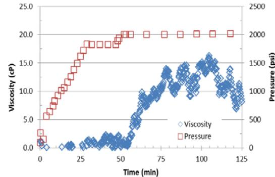
Viscosity of H<sub>2</sub>O-CO<sub>2</sub>-polymer mixture vs. pressure @ 190°C. Note: H<sub>2</sub>O-CO<sub>2</sub> viscosity: comparatively low, data not shown
