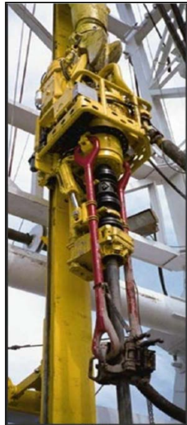
Top drive of rotary drill rig
