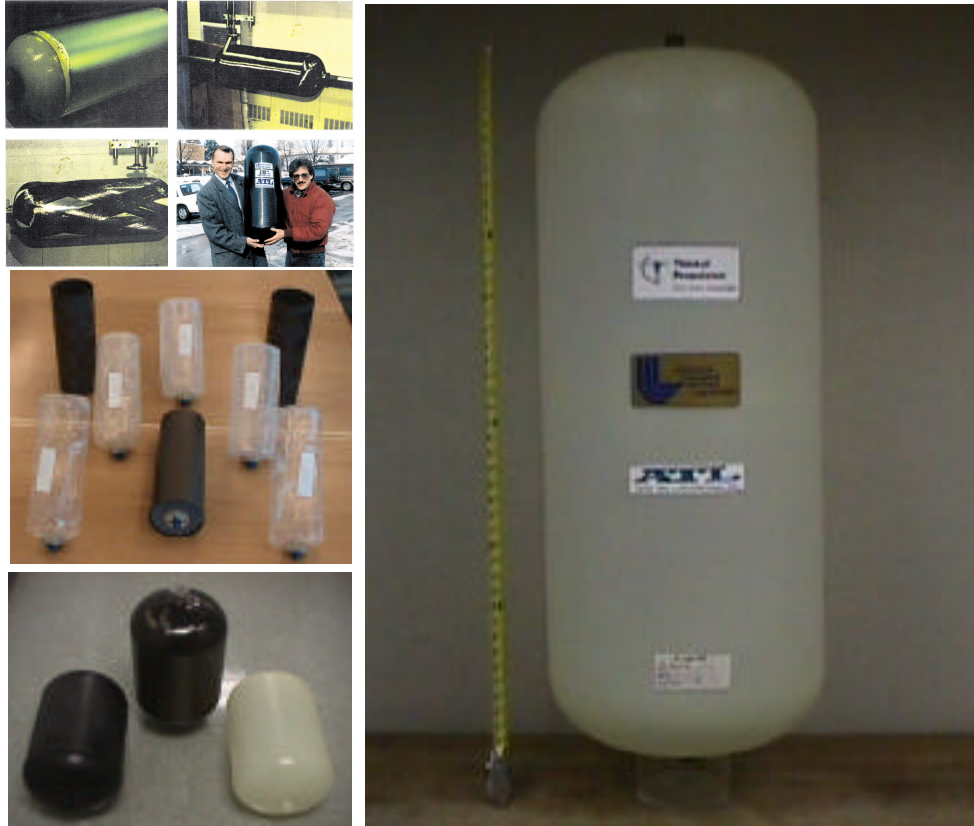
Figure 10 - Photos of LLNL/Thiokol/ATL Bladders and Tanks
