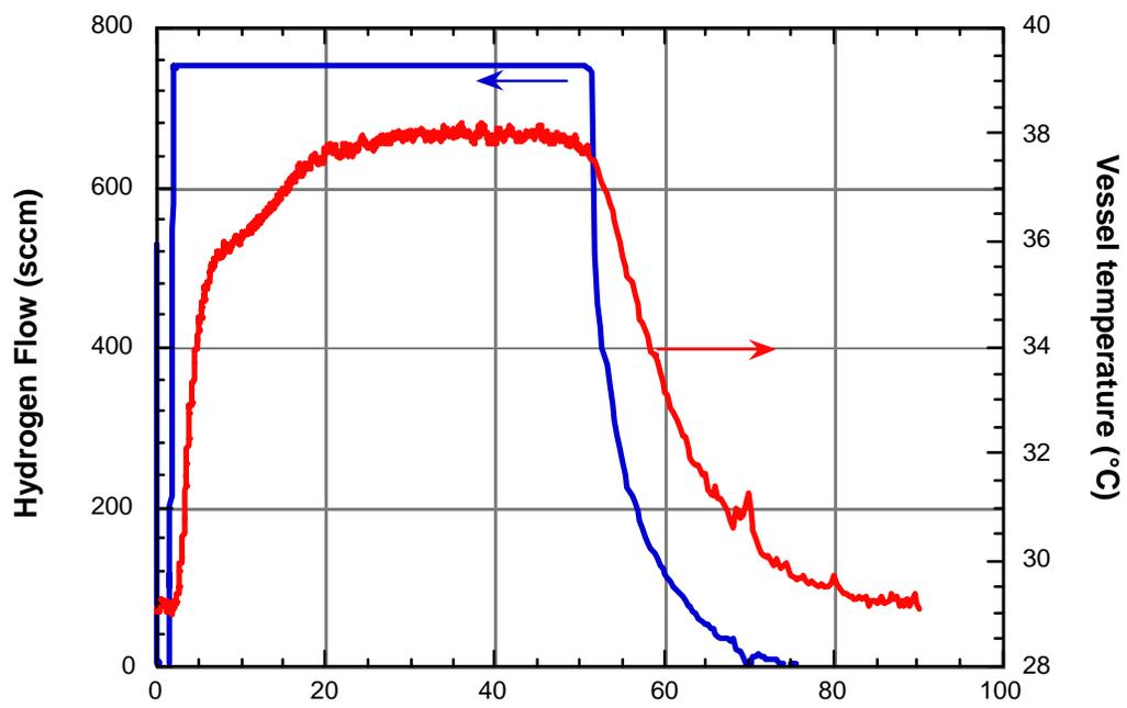
**Figure 5. Plots of hydrogen flow rate and bed temperature vs. time during filling of a hydride bed assembly.**
