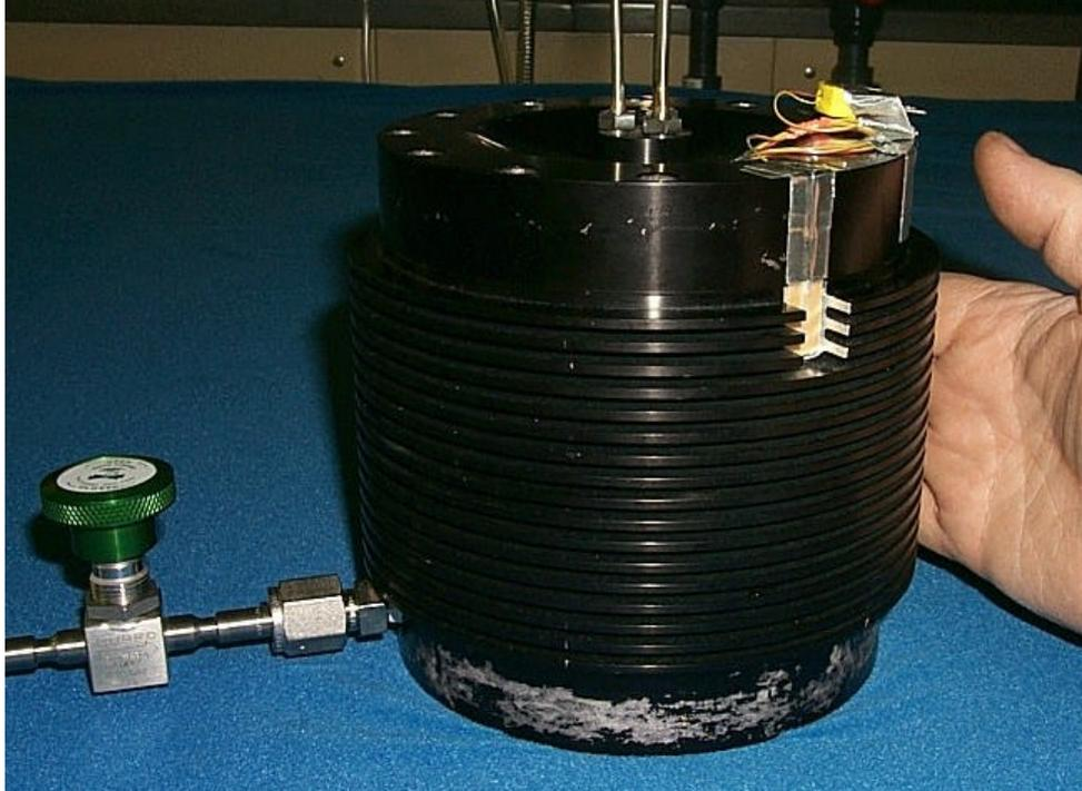
**Figure 1. A photograph of the hydride bed assembled for use in the laboratory at the University of Alaska, Fairbanks.**
