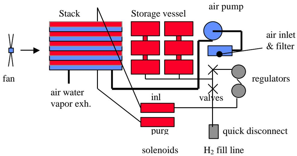
**Figure 3. An individual power assembly with a schematic diagram showing positions of components.**
