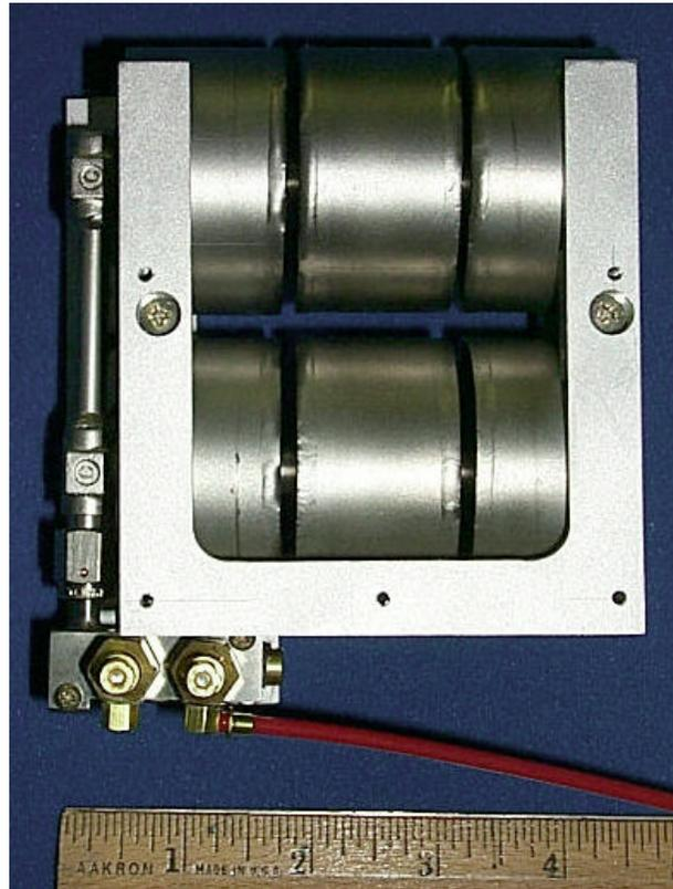
**Figure 4. One of the hydride bed assemblies.**
