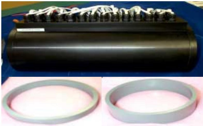
**Figure 7 – Magnequench Linear Alternator Stator Assembly**
