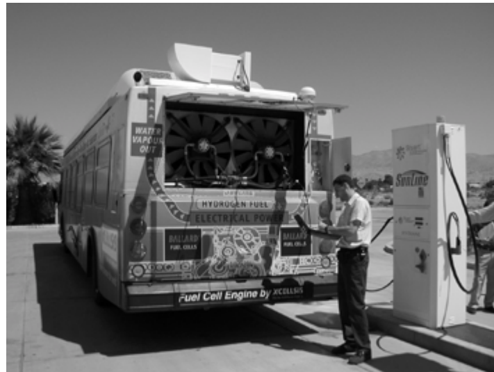
Figure 1. XCELLSiS field technician fueling the P4 bus with hydrogen
