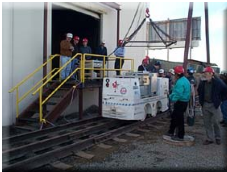
Figure 2: Fuel Cell Mining Vehicle to be fueled by P3-1B LP prototype.
