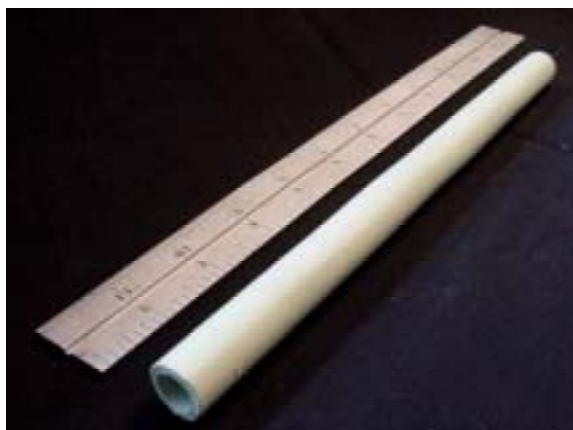
Figure 1: 12" long green tube, fabricated using the low pressure injection molding technique
