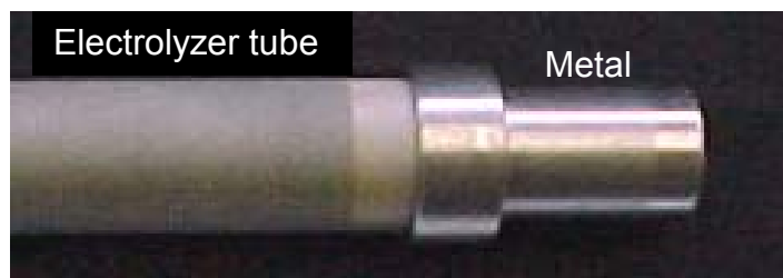
Figure 3: Picture of an electrolyzer tube sealed to a metal connector
