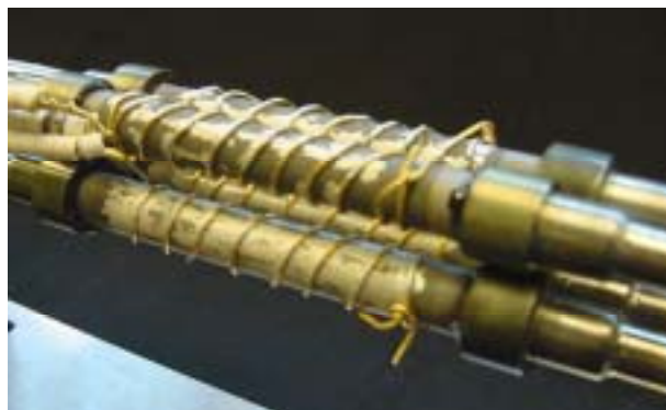
Figure 4: A 4-tube electrolyzer stack
