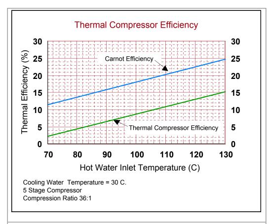
Figure 1 - Hydride "thermal" compressor operating efficiency is about 50% of Carnot efficiency.
