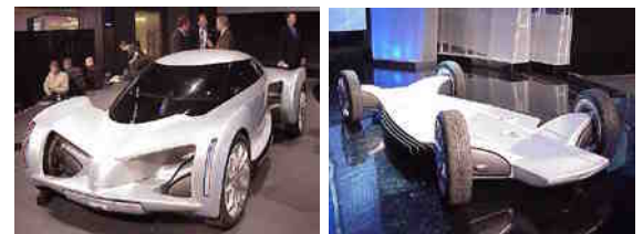
GM Autonomy Fuel Cell Car (left) and the “Skateboard” Platform (right)
