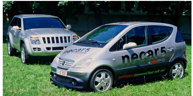
DaimlerChrysler NECAR 5 and Jeep Commander Fuel Cell Vehicles
