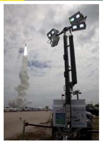
Hydrogen fuel cell powered light tower at Space Shuttle launch
