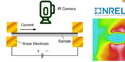
In-plane DC excitation/IR detection reveals bare spot in fuel cell electrode
