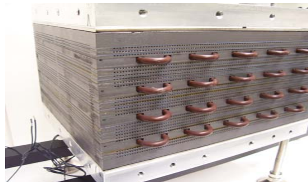
PBI 2KW Short Stack with 24 600cm 2 Cells
