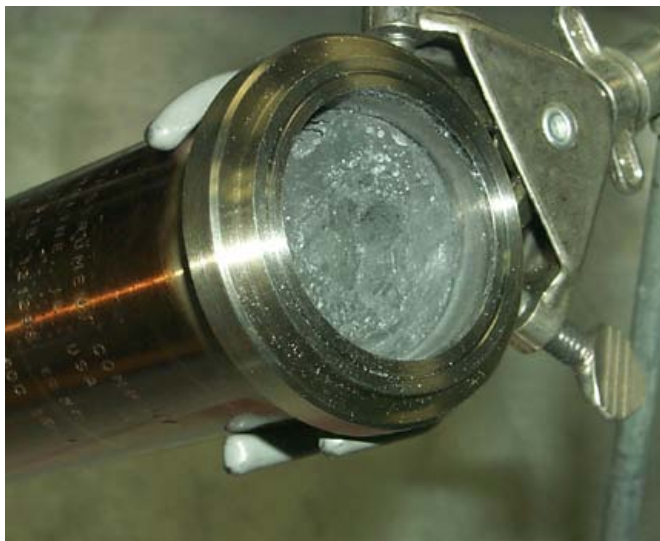
Figure 45. Scale up (100 g) reactor with end cap removed in Ar-glovebox to show catalyzed alanate. 69
