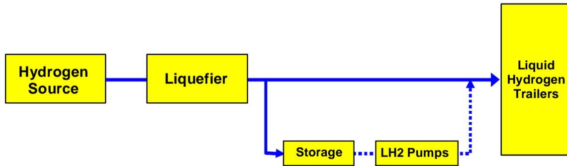
Figure 2-35 Liquid Terminal for Use with Gas Delivery
