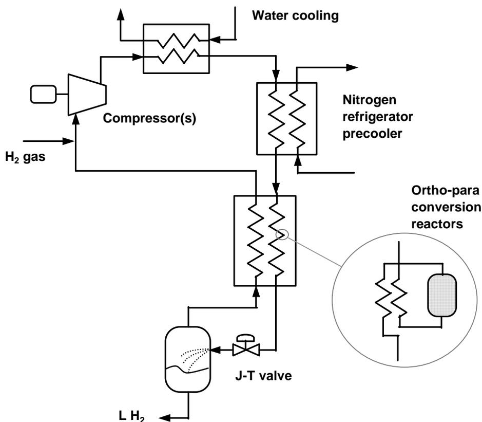
Figure 1-29 Simplified, pre-cooled Joule-Thomson cycle for hydrogen liquefaction
