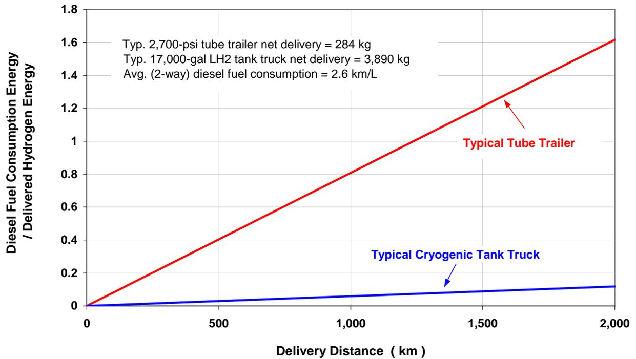
Figure 1-28 Diesel fuel consumption energy relative to delivered hydrogen energy for different tube trailer and cryogenic tank truck delivery distances.
