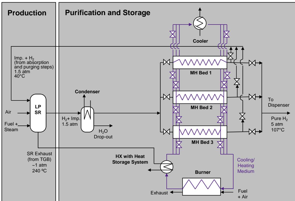
Figure 1-40 Dry Metal Hydride Based Hydrogen Separation from Reformate Stream
