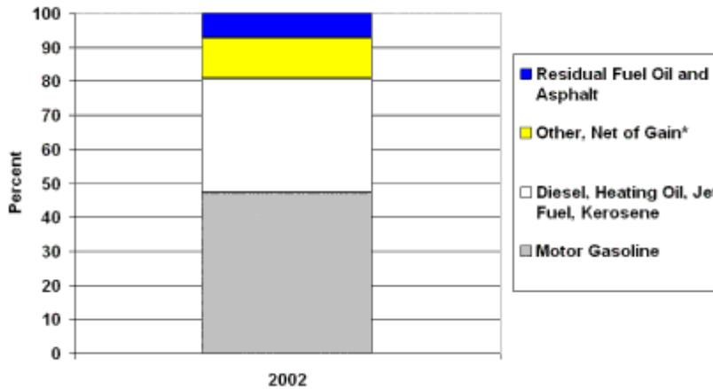
Figure 1-22 Average US Refinery Outputs from Crude Oil
