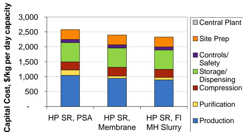
Figure 1-43 Capital Cost for Steam Reformer Central Plant with Hydrogen Purification
