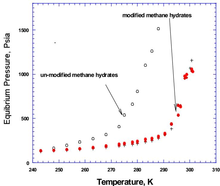
Figure 1-35 Equilibrium Pressure vs. Temperature Curve of Methane Hydrate with New Additive
