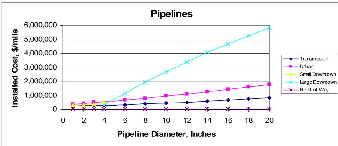
Figure 2-12 Compilation of Steel Pipeline Unit Cost Data
