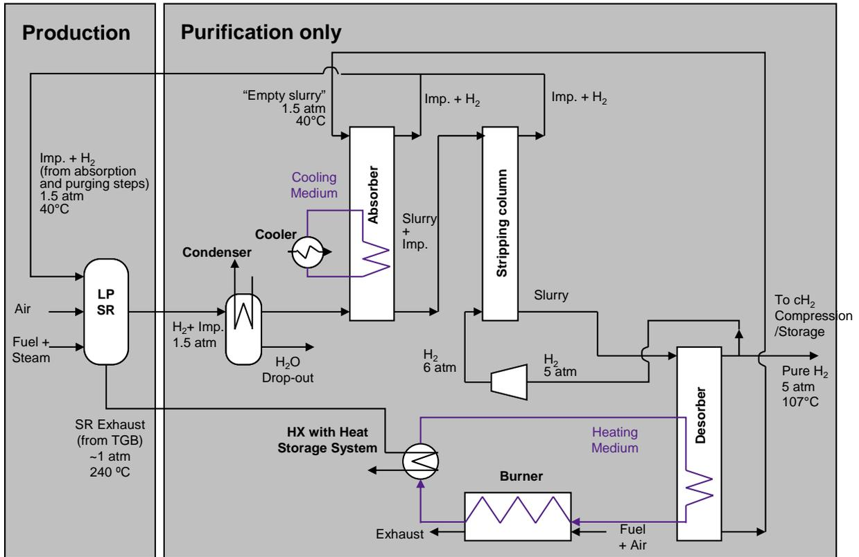
Figure 1-41 Metal Hydride Slurry Based Hydrogen Separation from Reformate Stream
