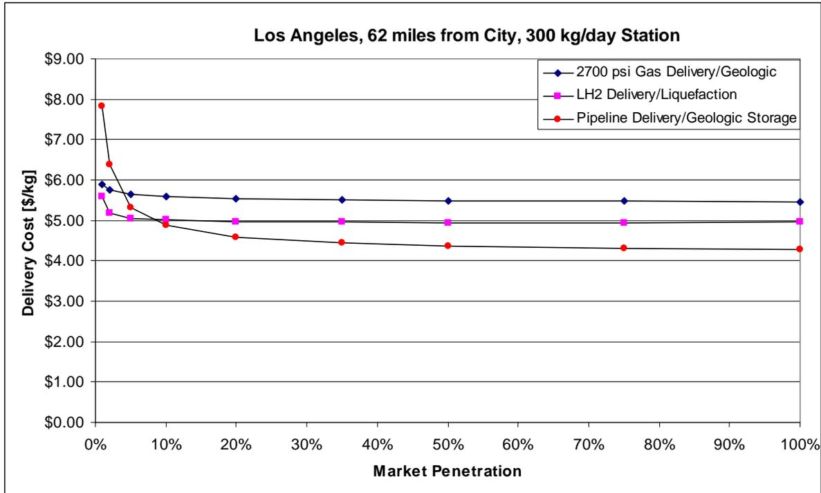
Figure 3-9 Comparison of Delivery Modes for 300 kg/day Stations
