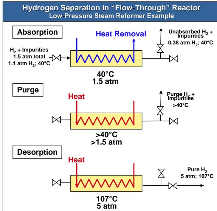
Figure 1-39: Schematic Representation of Metal Hydride Based Hydrogen Purification
