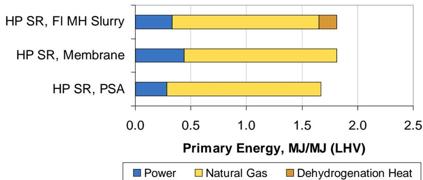
Figure 1-42 Primary Energy Requirement for H<sub>2</sub> Separation from HP SR Reformate Streams
