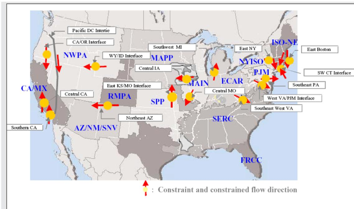
Figure 1-56 Overview of Transmission Constraints in the US
