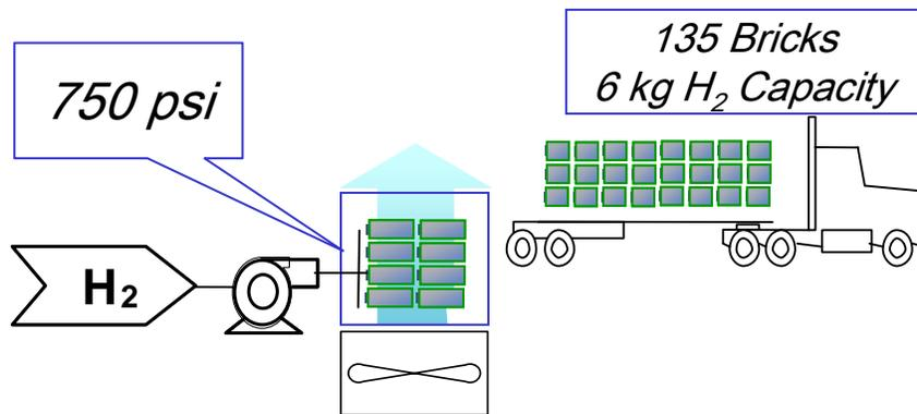
Figure 1-32 Hydrogen Brick Delivery System
