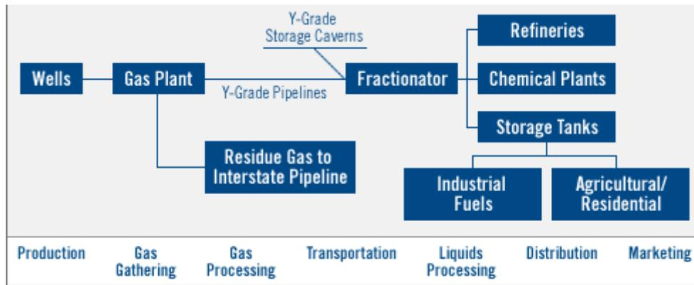
**Figure 1-2 Natural Gas Production and Distribution System**
