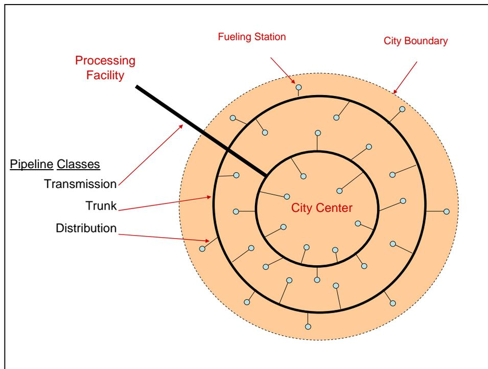
**Figure 5: Simplified Pipeline Diagram**
