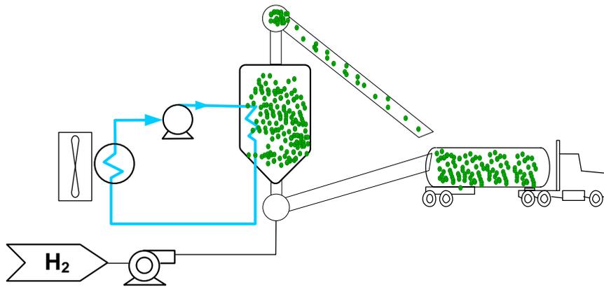
Figure 1-33 Illustration of flowable powder processing, including H<sub>2</sub> compression and heat removal
