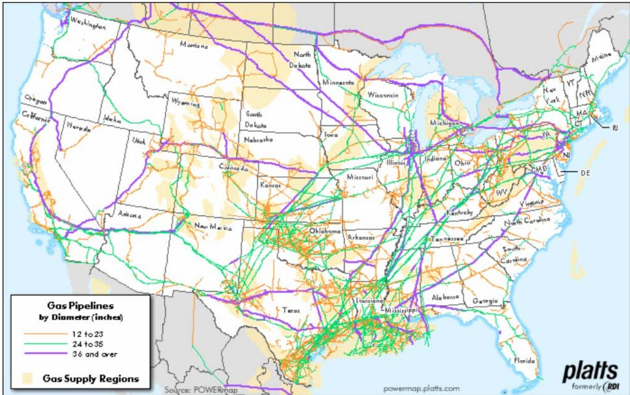
Figure 1-3 Principal Domestic Natural Gas Transmission Pipelines
