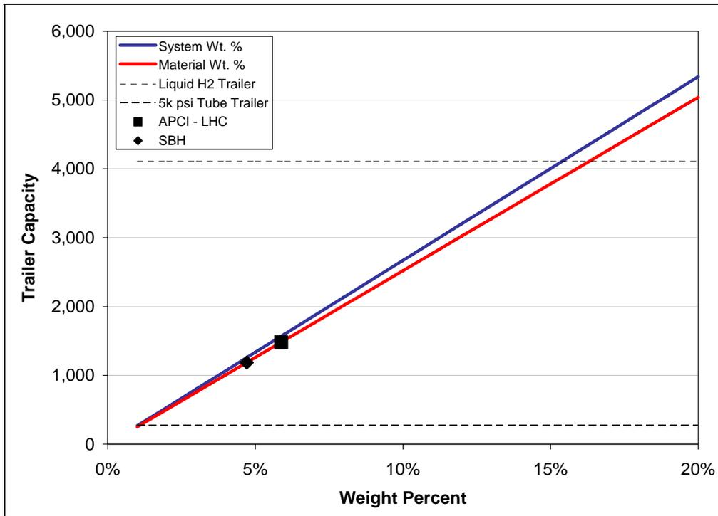
**Figure 1: Novel Hydrogen Carrier Truck Capacity (kg)**
