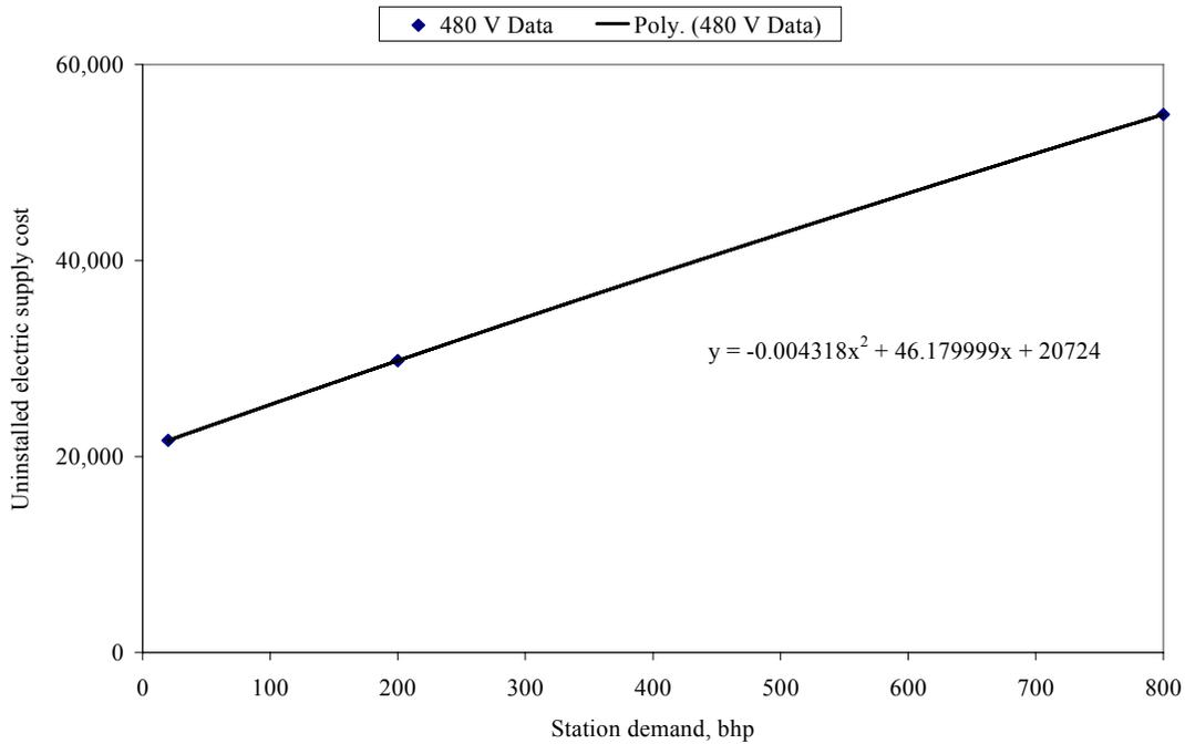
Figure 2-26 Refueling Station Electric Supply Costs - 480 Volts
