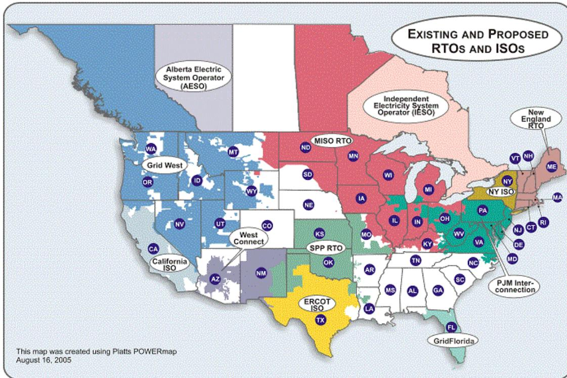
Figure 1-53 Federal Energy Regulatory Commission Map of Regional Transmission Operators and Independent System Operators
