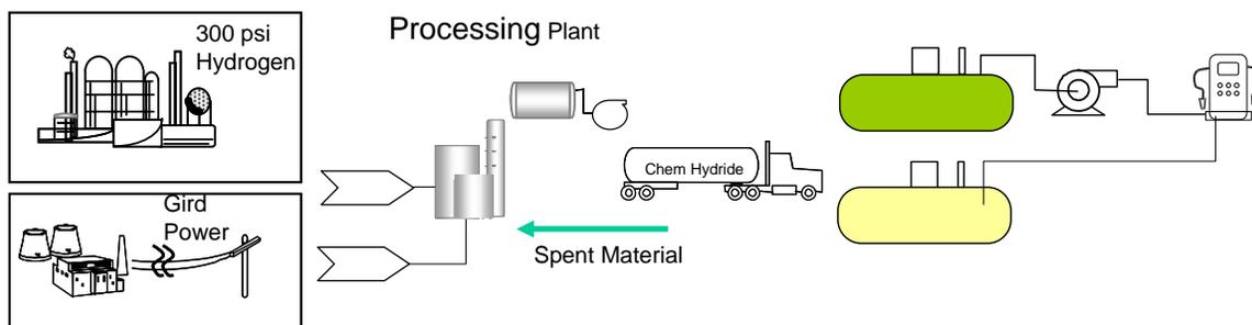
Figure 1-31 Chemical Hydride Processing and Delivery System
