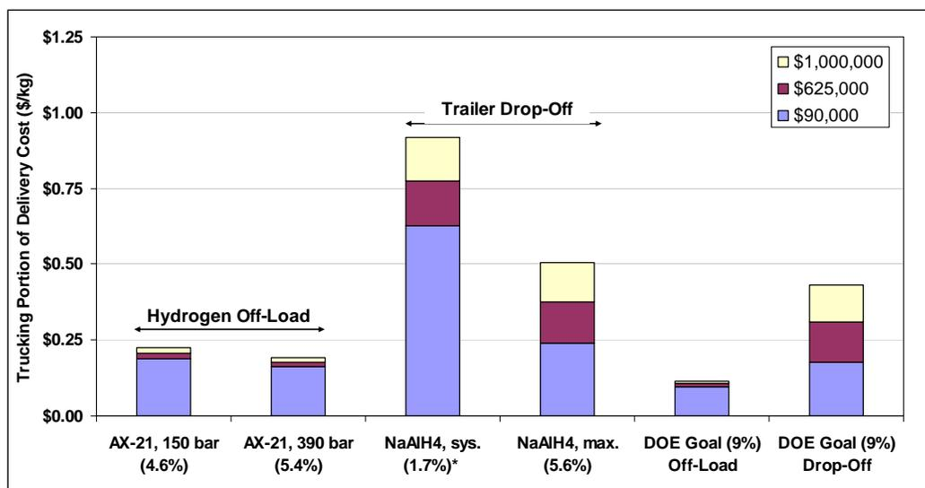
**Figure 4: Solid-State Hydrogen Trucking Cost**
