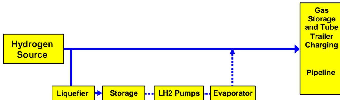
Figure 2-36 Liquid Terminal for Use with Gas Delivery
