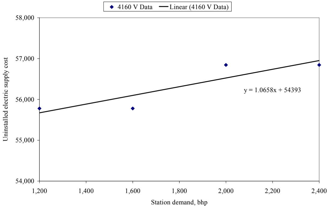
Figure 2-27 Refueling Station Electric Supply Costs - 4160 Volts
