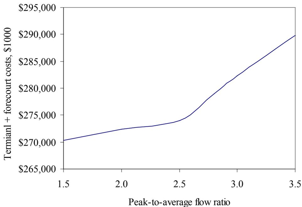
Figure 2-19 Gas Terminal and Refueling Station Cost Estimates
