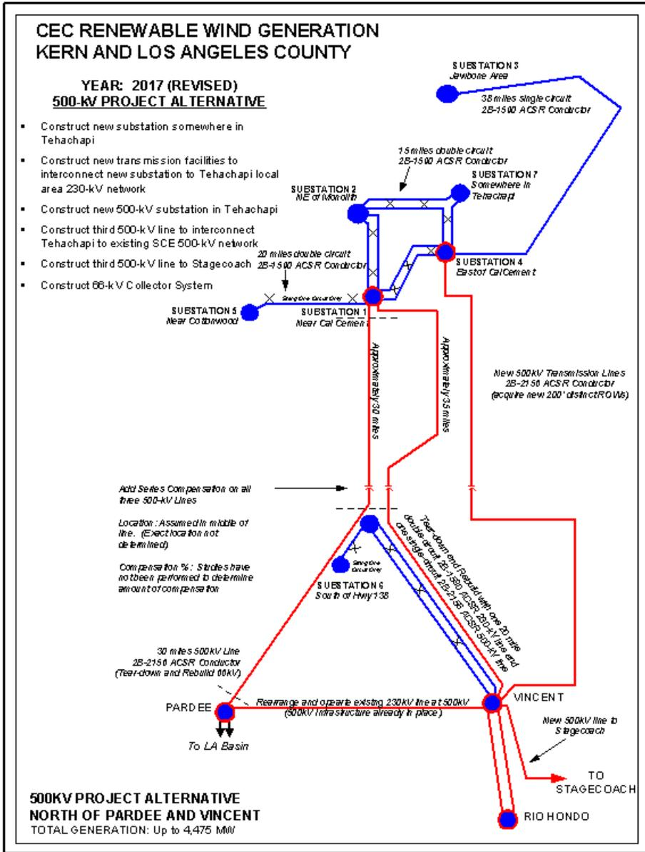
Figure 1-54 Possible Expansion Scenario for One Segment of the California Transmission System
