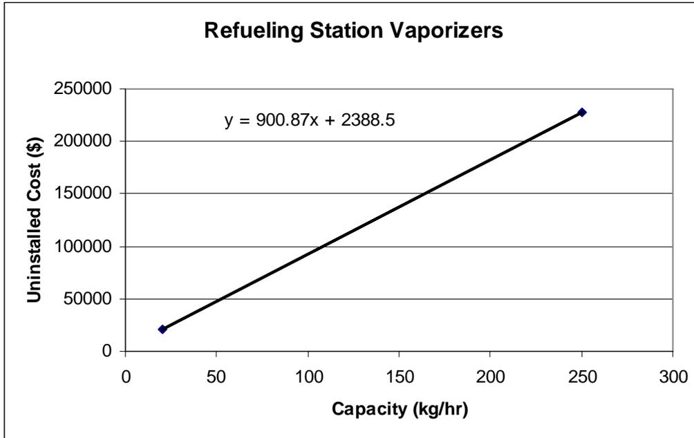
Figure 2-33 Uninstalled Costs for Refueling Station Hydrogen Vaporizers
