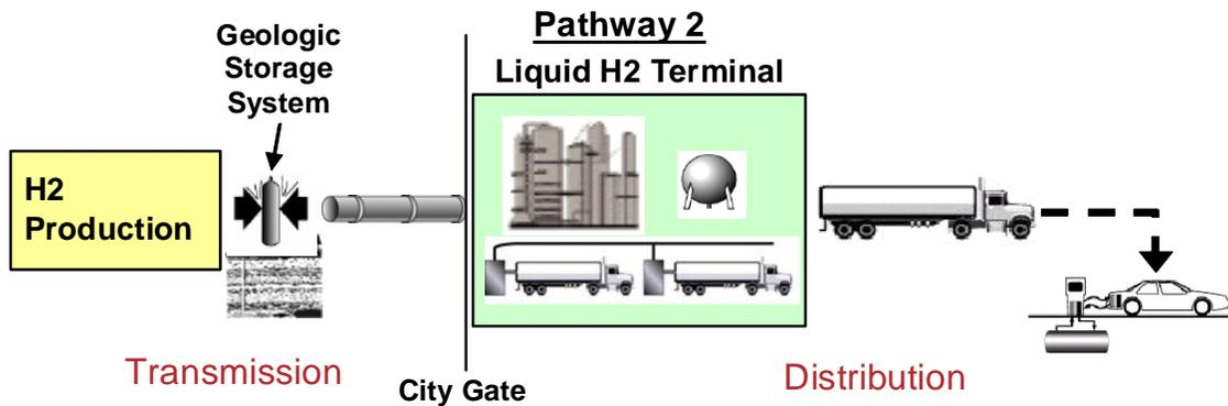
Figure 0-4 Pathway 2: Mixed Mode Liquid Delivery Pathway with Long Term Geologic Storage
