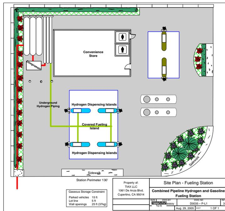
Figure 2-40 Pipeline Supplied Fueling Station Site Plan
