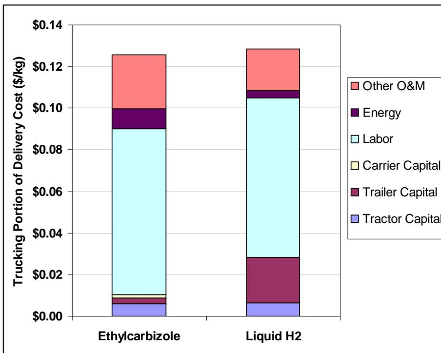
**Figure 3: Cost Breakdown of Ethylcarbizole and Liquid H2 Trucking**
