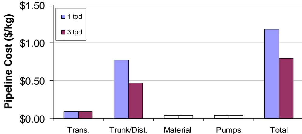
**Figure 6: Pipeline Delivery Cost Breakdown**
