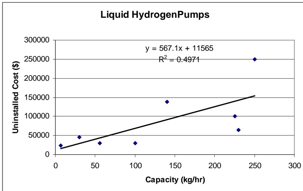
Figure 2-32 Uninstalled Costs for Liquid Hydrogen Pumps
