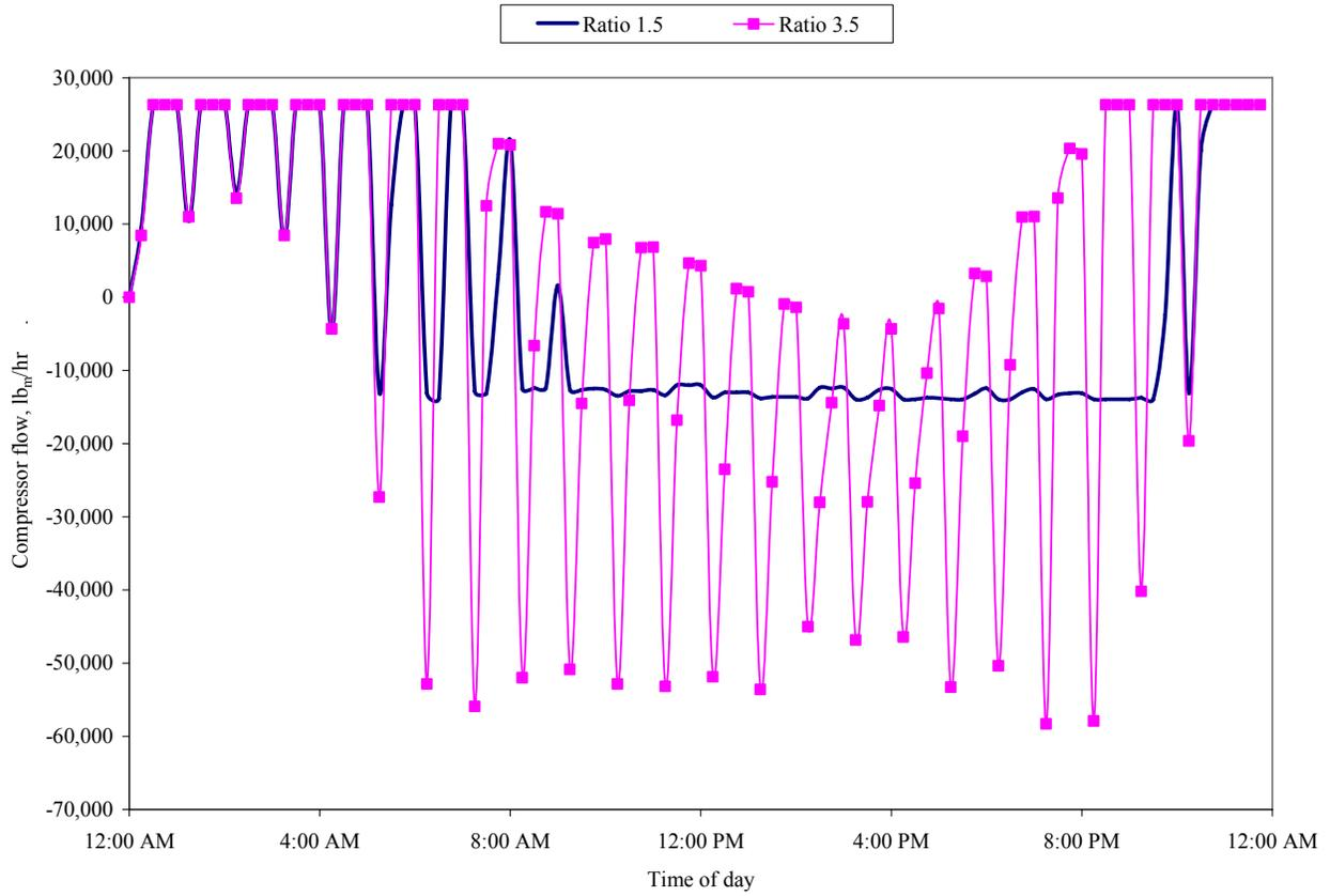
Figure 2-18 Gas Terminal Compressor Flow Demand
