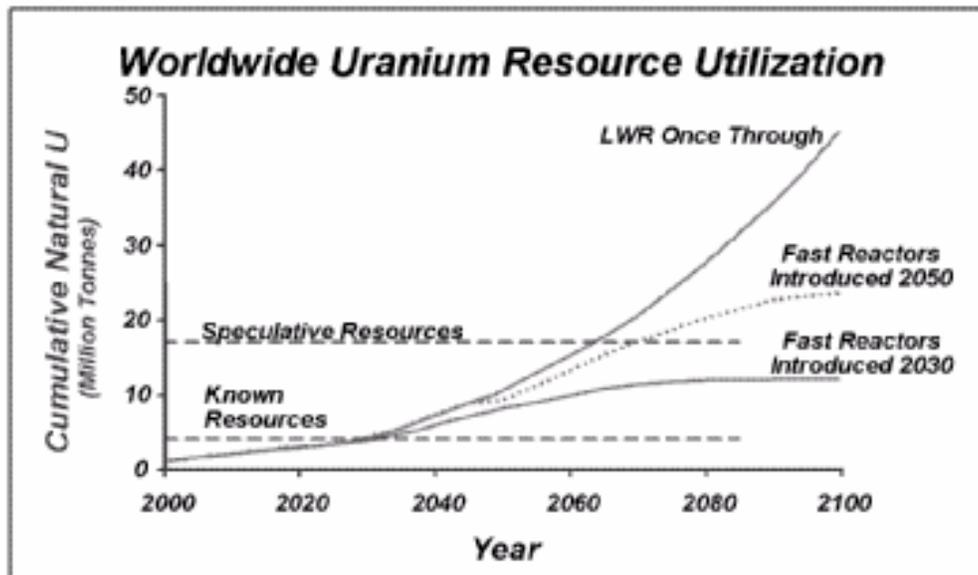
Figure 1-16 Cumulative Uranium Consumption and Resources
