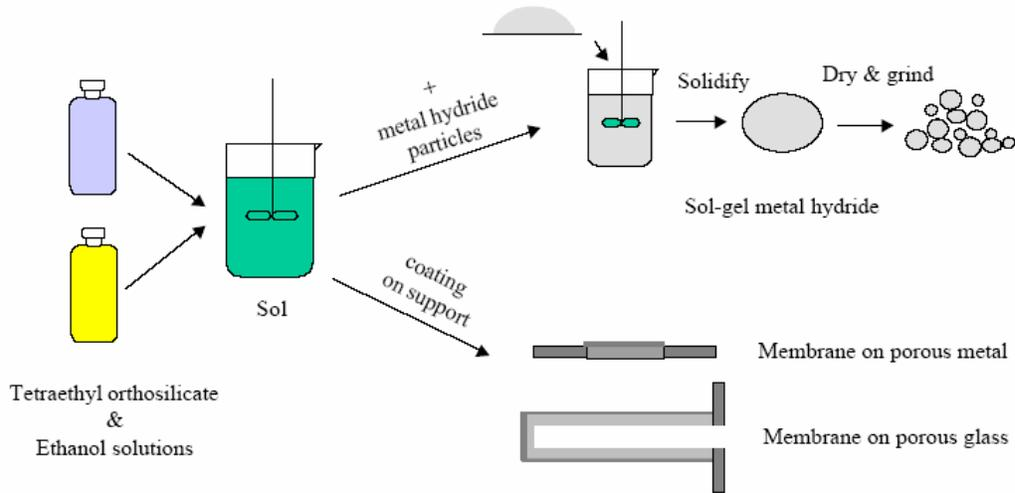
Figure 1-37 Schematic of Sol-Gel Metal Hydride and Sol-Gel Membrane Process
