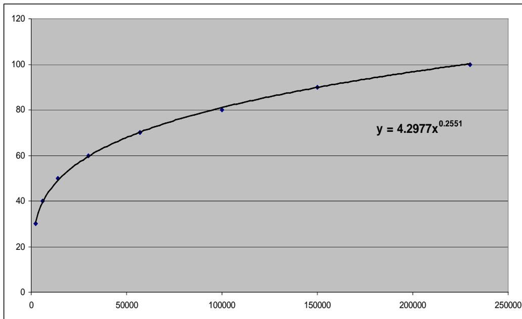
**Figure 2-11 Labor Cost as a Function of Capacity (vertical axis: relative labor cost; horizontal axis: system capacity in kg/hour) <sup>27</sup>**
