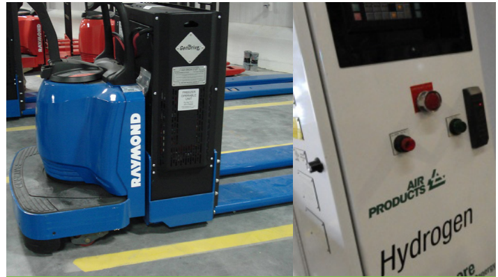
Left: Class III fuel cell powered lift truck at Sysco Houston distribution center in Houston, TX. Sysco Houston. Right: Indoor refueling station for fuel cell powered lift trucks at FedEx Freight East facility in Springfield, MO. FedEx Freight East.
