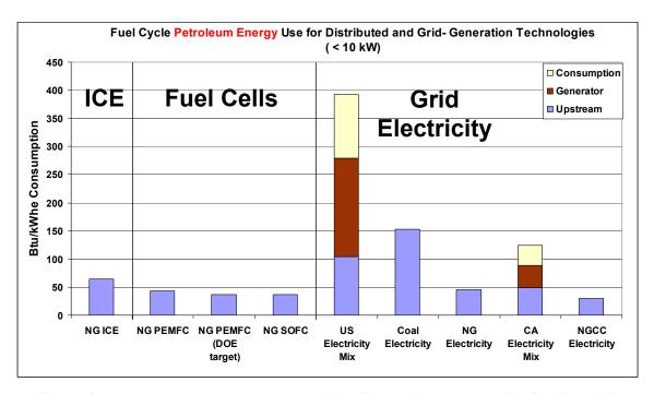
FIGURE 4. Petroleum Energy Use by Electricity Generation Technologies for Capacities  $\,<\,10~kW$
