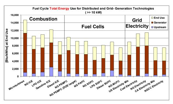
FIGURE 6. Total Energy Use by Electricity-Generation Technologies for Capacities  $>> 10~\mathrm{kW}$
