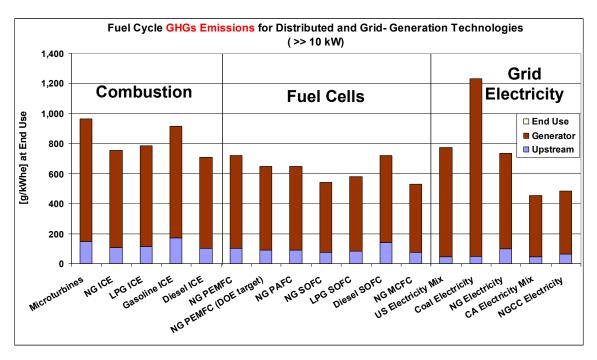
FIGURE 9. GHGs Emissions by Electricity-Generation Technologies for Capacities  $>> 10\;\mathrm{kW}$
