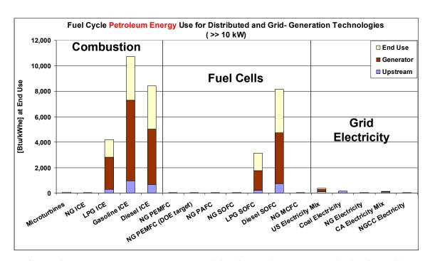
FIGURE 8. Petroleum Energy Use by Electricity-Generation Technologies for Capacities >> 10 kW
