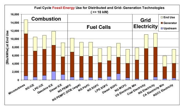
FIGURE 7. Fossil Energy Use by Electricity-Generation Technologies for Capacities  $>> 10\;\mathrm{kW}$
