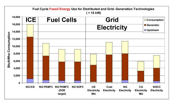
FIGURE 3. Fossil Energy Use by Electricity Generation Technologies for Capacities  $\,<\!10~kW$
