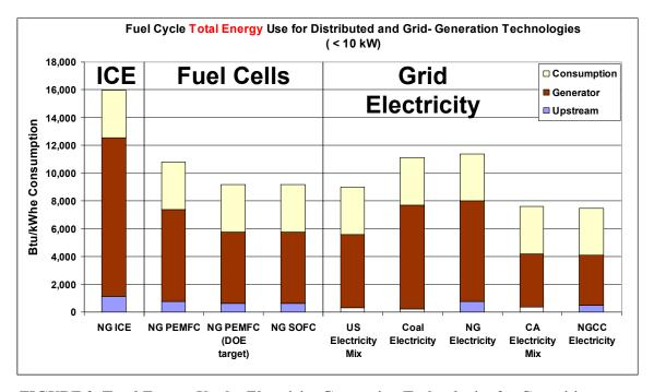
FIGURE 2. Total Energy Use by Electricity Generation Technologies for Capacities  $\,<\,10~kW$
