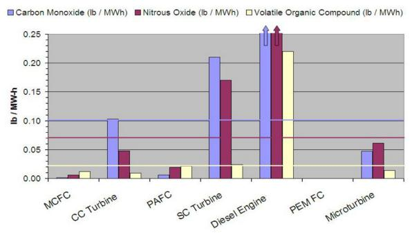
FIGURE 1. Criteria Pollutants Emissions for Distributed Generation Technologies (Source: Tollstrup 2008)
