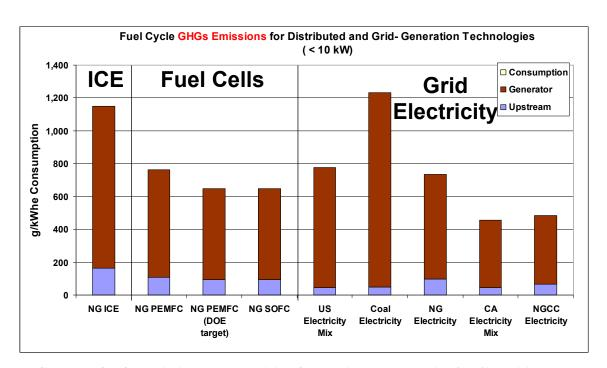
FIGURE 5. GHGs Emissions by Electricity Generation Technologies for Capacities  $\,<\,10~kW$
