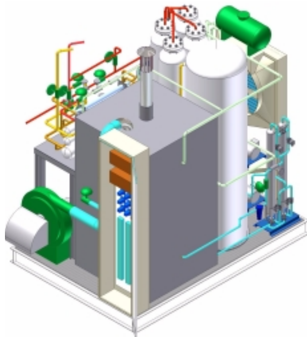
Figure 3. Low-Cost Hydrogen Production Platform - Skid Cover Off
