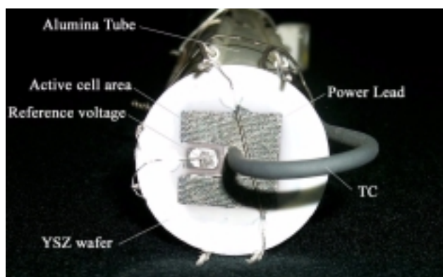
Figure 1. Details of Solid-Oxide Button Cell Fabricated by Ceramatec (TC = thermocouple, YSZ = yttria-stabilized zirconia)
