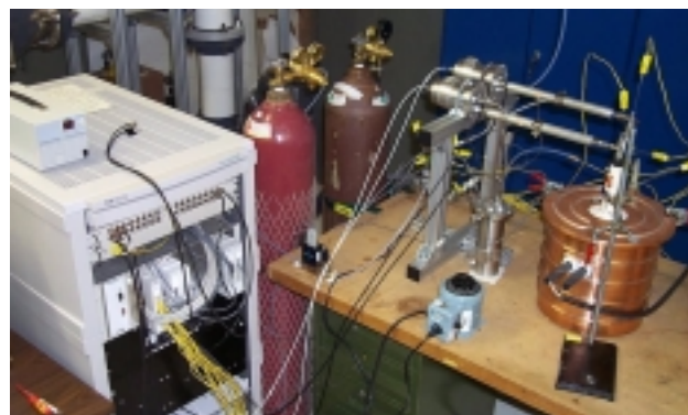
Figure 2. High-Temperature Single-Cell Steam Electrolysis Test Setup at INEEL
