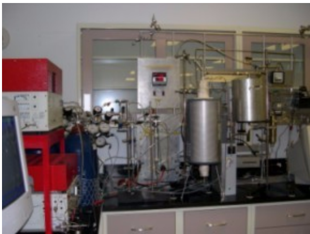
Figure 2. Experimental Set-up with 3-kW th Thermocatalytic Reactor
