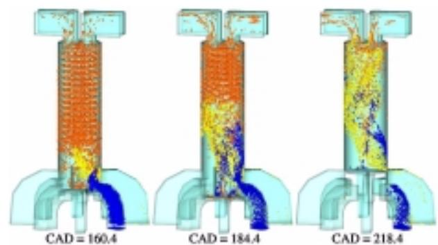
Figure 3. Calculated Stratified-Scavenging Flows
