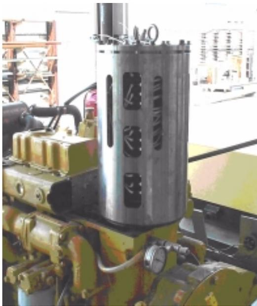
Figure 2. Alternator Test Rig
