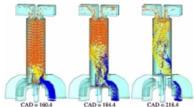
Figure 3. Calculated Stratified-Scavenging Flows
