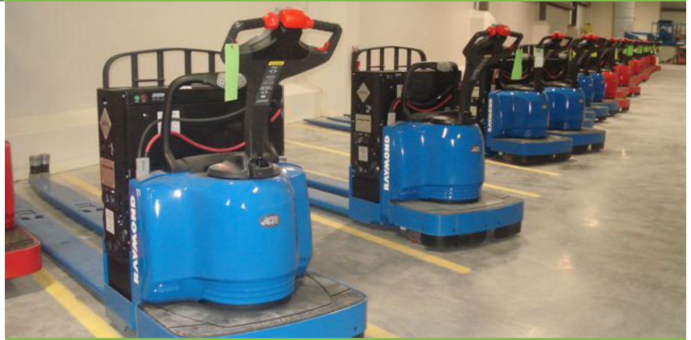
Class III fuel cell powered lift truck at Sysco Houston distribution center in Houston, Texas. Sysco Houston.
