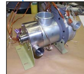
Demonstration of Motor Driven Turbocompressor w/Mixed Flow Compressor and Variable Nozzle Turbine DoE 50kW PEM Fuel Cell System for Light Duty Vehicle 2001
