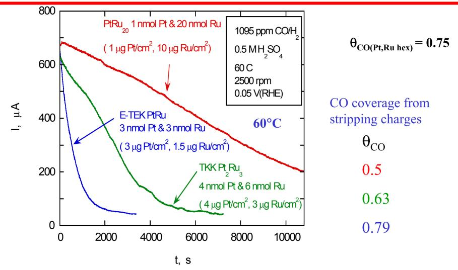
Lower Pt-CO bond strength and an efficient CO spillover to RuOH are likely cause of enhanced CO tolerance.
