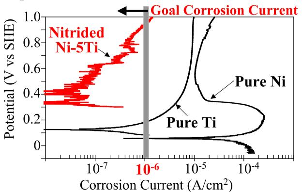
•BUT issues remain with poor reproducibility and local corrosion attack at edges and some nitride surface sites(?)
