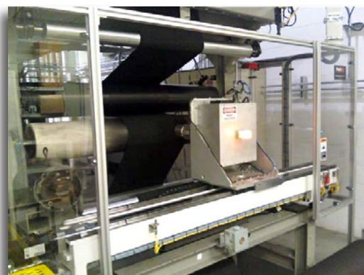
*BASF's High-Speed Coating Machine with XRF Monitoring*
