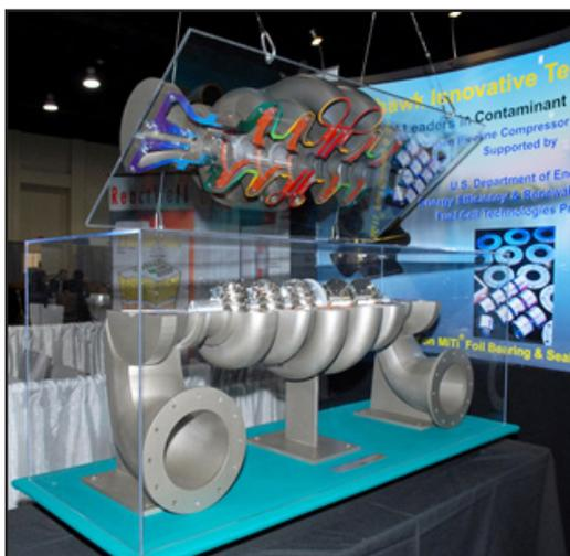
Full Scale Mockup of MiTi Hydrogen Compressor
