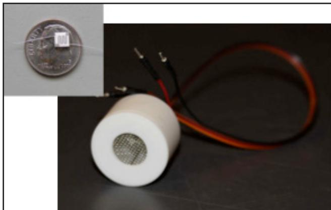
*Packaged Electrochemical H<sub>2</sub> Safety Sensor*
