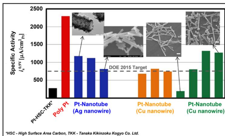
NREL's Pt Electrode Nanostructured Technology
