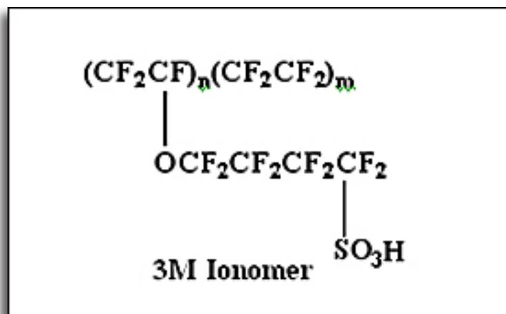
*The 3M Ionomer With Lower Equivalent Weight Side Chain than Standard PFSA Ionomers*
