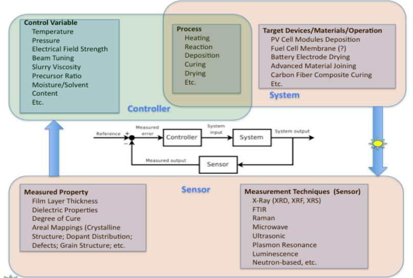
In some cases, e.g. microwave processing, the system can act as the "sensor" (by monitoring and controlling forward and reflected power).
