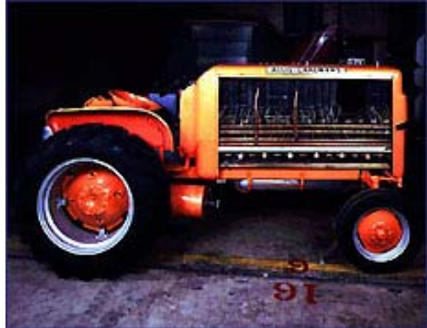
Allis Chalmers fuel cell tractor, 1959
