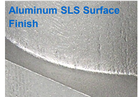
Aluminum SLS Part Post Machining
