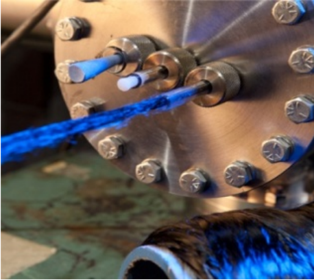
Carbon Fiber exiting Microwave Assisted Plasma (MAP) process
