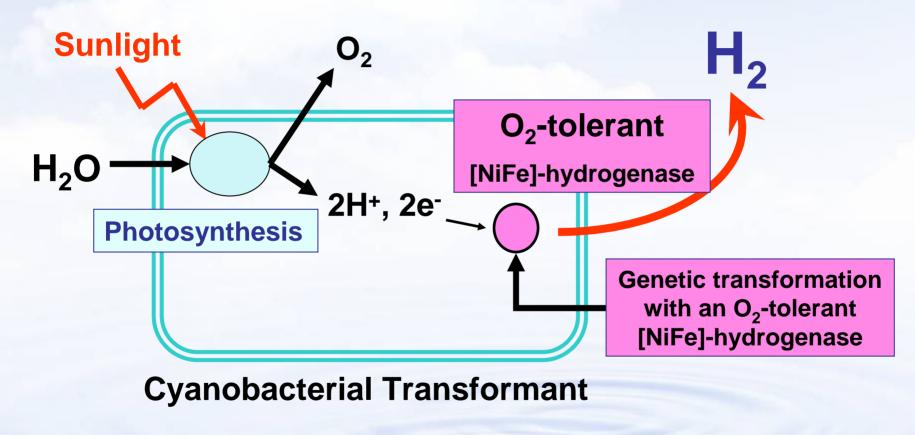
An O<sub>2</sub>-tolerant [NiFe]-hydrogenase has been identified from the photosynthetic bacteria, *Rubrivivax gelatinosus* and *Thiocapsa roseopersicina*. This O<sub>2</sub>-tolerant [NiFe]-hydrogenase will be genetically expressed in a cyanobacterium for continuous photo-production of H<sub>2</sub> and O<sub>2</sub> from water.
