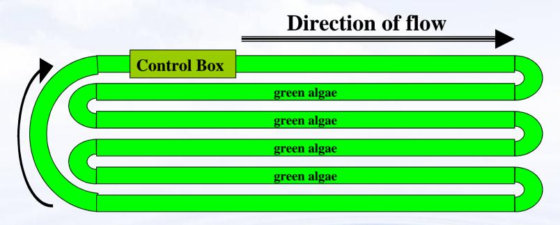
Example of an enclosed, tubular racetrack, low-cost photobioreactor for photosynthetic microorganism growth, H<sub>2</sub>-production, and H<sub>2</sub>-gas harvesting. Depending on the optical properties of the cells (e.g. Barrier X), the tube diameter would be 6-12 inches wide. Other reactor configurations are possible, depending on climatic and local conditions.
