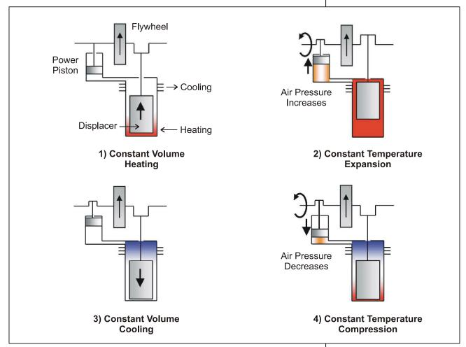
Figure 8-9 Stirling Engine Operation
