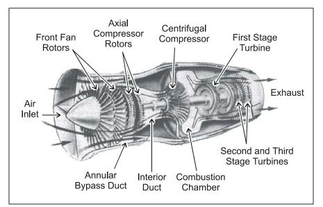
Figure 8-10 Gas Turbine Engine Major Components
