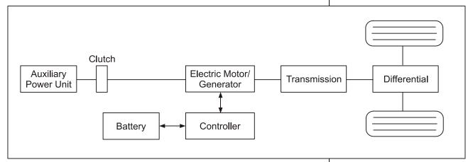
Figure 8-3 A schematic of a Parallel HEV
