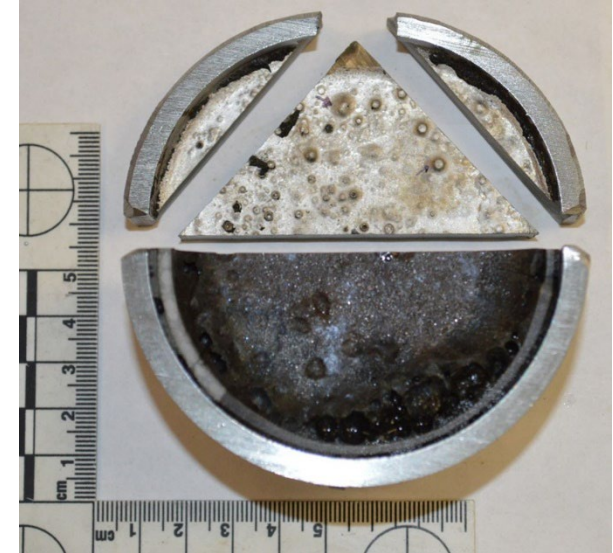
Iron deposited during laboratory-scale MOE experiment
