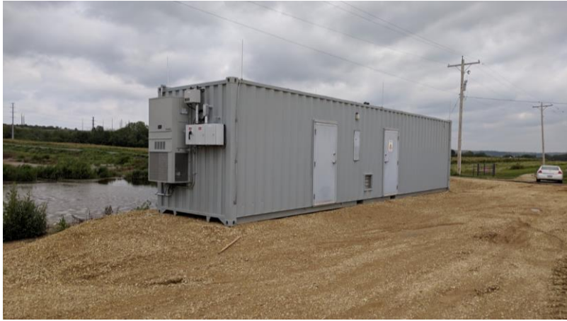
Pilot AnMBR unit at K-State (1000 gpd)
