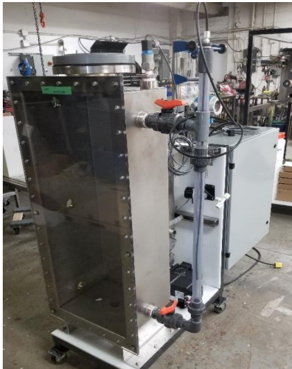
Pilot AnMBR unit at K-State (1000 gpd)
