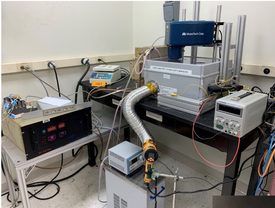
RF/US/ Convection drying experimental setup
