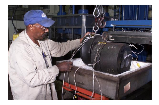
The entire tool stack was heated from one side with our existing 88 kW furnace at ORNL. As seen, the dies are much too large to fit in the existing setup.
