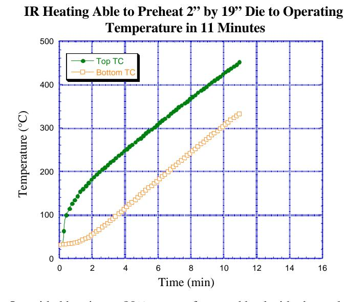
One sided heating at 80% power, front and back side thermal couples
