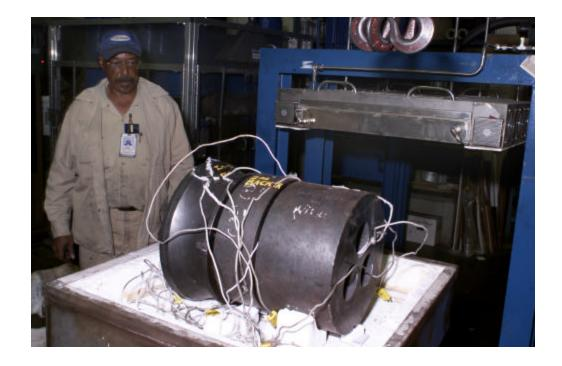
The entire tool stack was heated from one side with our existing 88 kW furnace at ORNL with some modification to accommodate the large dies..
