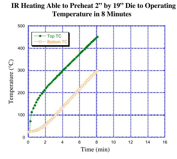
One sided heating at 90% power, front and back side thermal couples
