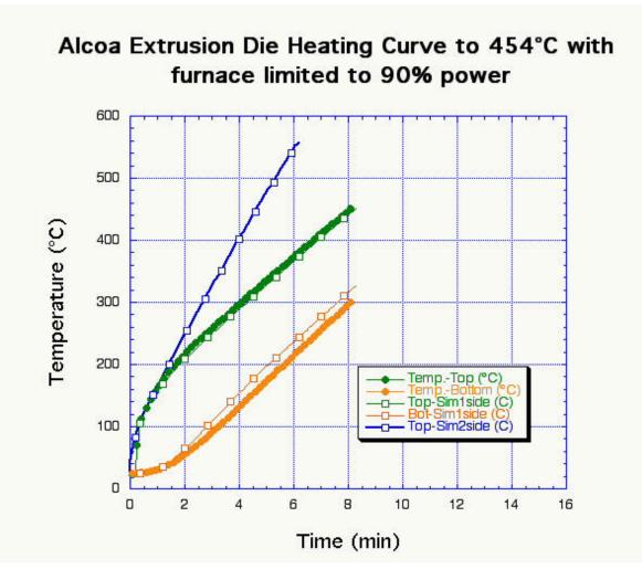
Experimental one sided heating at 90% power, front and back side thermal Couples, modeled front and back side, and modeled two sided heating, 2" thick by 19" diameter die.
