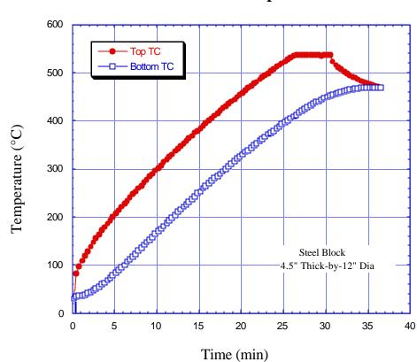
Steel Block Heating Curve to 537°C with furnace limited to 70% power
