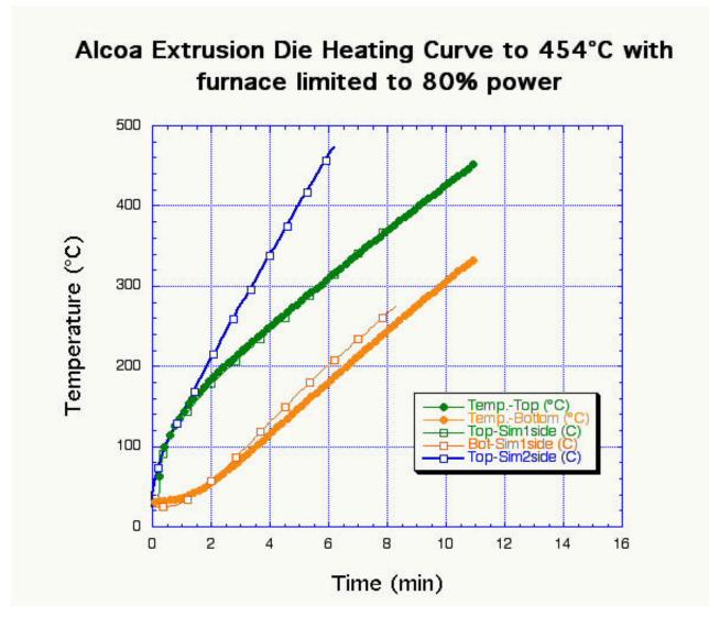
Experimental one sided heating at 80% power, front and back side thermal Couples, modeled front and back side, and modeled two sided heating, 2" thick by 19" diameter die.
