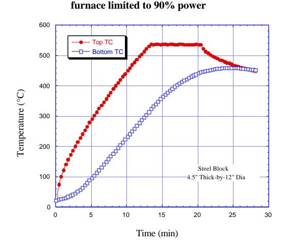
**Steel Block Heating Curve to 537°C with**
