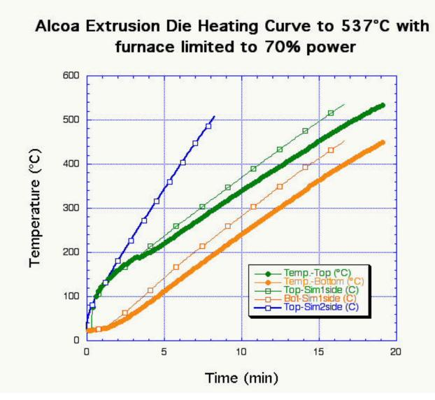
Experimental one sided heating at 70% power, front and back side thermal Couples, modeled front and back side, and modeled two sided heating, 2" thick by 19" diameter die.
