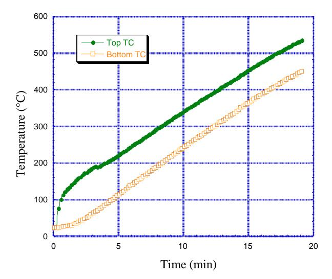
One sided heating at 70% power, front and back side thermal couples
