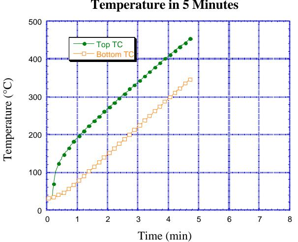
IR Heating Able to Preheat 1" by 12" Die to Operating Temperature in 5 Minutes
