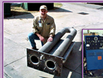
Nickel aluminide radiant burner installed at Weirton Steel Corporation
