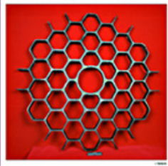
IC221M Grid Prior to Installation in Carburizing Furnace at Timken
