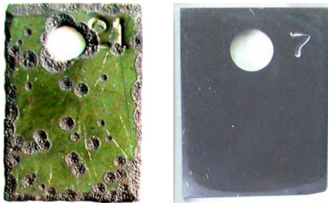
Figure 3. Photograph of commercial Ni-base Alloy 600 and ANL-developed alloy after 5,700-h exposure to the same metal dusting environment at 593°C.
