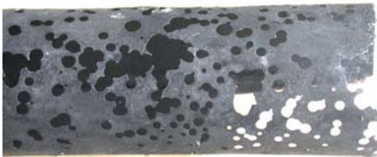
Figure 1. An alloy tube from a syngas plant that has been severely damaged by metal dusting.
