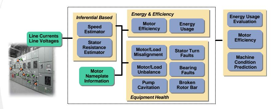
No speed and torque sensors needed? Inferential, non-intrusive, low-cost!
