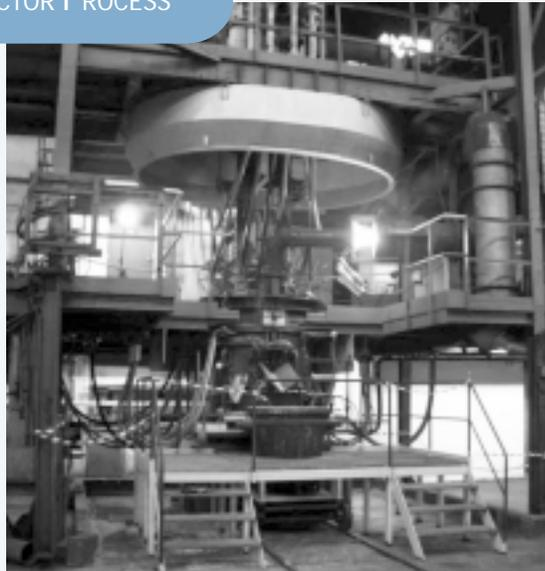
**ARP is a new process for producing aluminum.**
