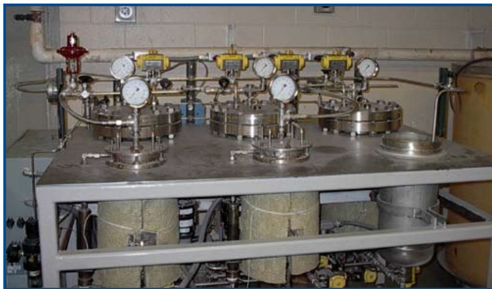
Profiling digester system used for pre-extraction of wood chips.
