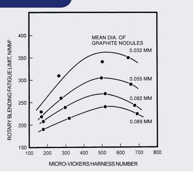
Correlation of fatigue strength with graphite nodule size in ductile irons of varying matrix hardness.
