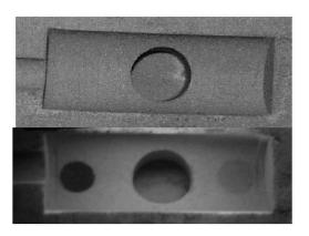
**U**pper image shows a mold containing 3 and 5% lower density areas that are normally invisible. Under certain conditions, the lower image shows that these lower density areas can be visualized. This tool will allow molds/cores to be discarded or modified <u>before</u> casting takes place, thus eliminating considerable cleaning room time.
