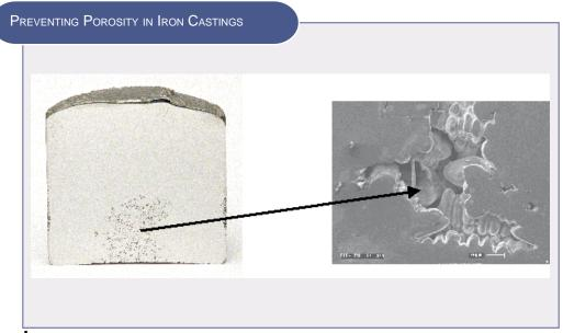
Interdendritic porosity in a Ni-Hard I casting melted and solidified under 1 atm nitrogen pressure.
