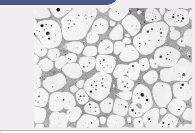
This special microstructure gives semi-solid metal its unique advantage. When heated to the "mushy" state, the material flows as a fluid, but retains other solid-like behaviors.
