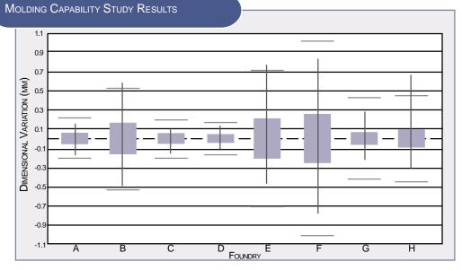
Foundry test results. Lines represent (+, -) three sigma deviations.
