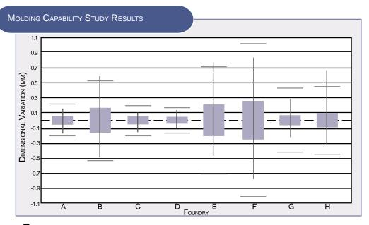
Foundry test results. Lines represent (+, -) three sigma deviations.
