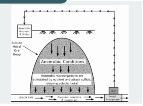
Geo-Microbial Technologies' anaerobic bioleaching technology uses anaerobic cultures to remove metal values from ore at lower costs and without great environmental impact.
